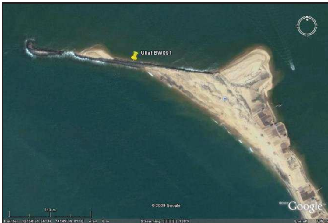
Figure 8: Nethravathii-Gurupura Estuary during 2009, the Breakwater Started Collapsing.
