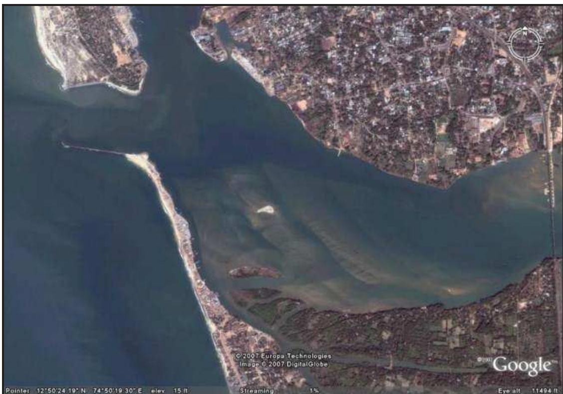
Figure 6: Nethravathi - Gurupura Estuary during 2007. Siltation and Sand Bars are Noticed on the Southern Side of the Estuary (Courtesy: Google Earth)
