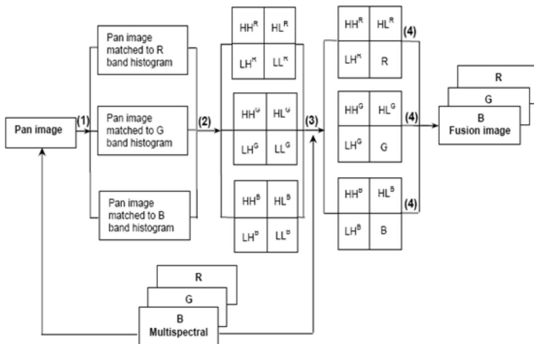
**Fig.3** The DWT algorithm
