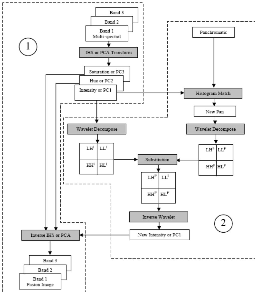
**Fig.5: Basic steps for IHS method for wavelet transform.**
