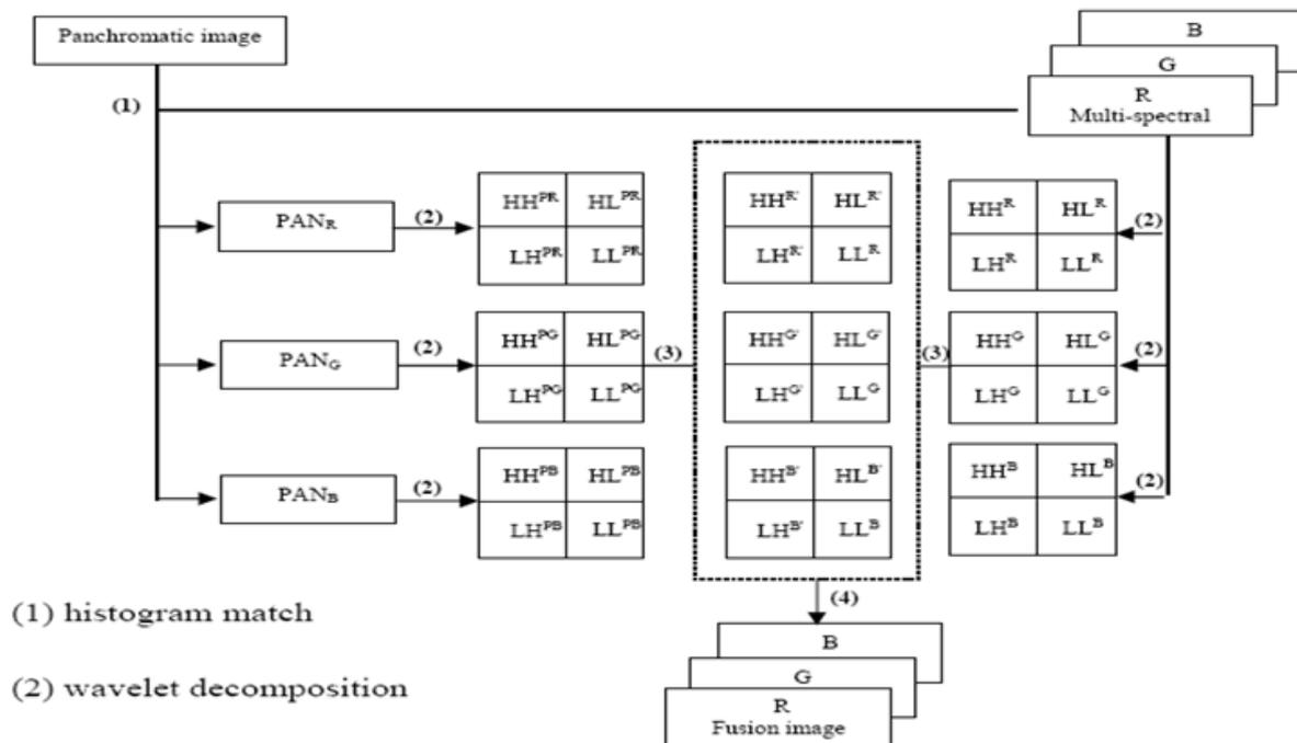
Fig.4 Schematic diagram of additive wavelet based image.
